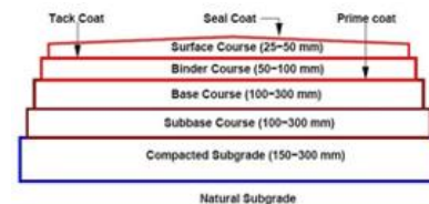
Fig. 1. Typical cross section of a flexible pavement
