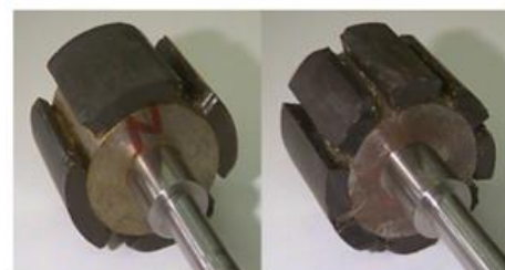
Fig. 2. 4-pole and 8-pole permanent magnet rotor
