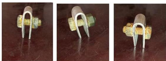
Fig. 3. Photograph of the samples S1, S2, S3 respectively after SCC testing
