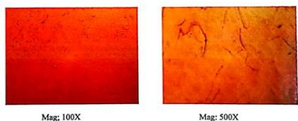
Fig. 5. Microstructure of sample S2 (shot peened)
