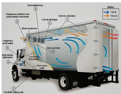
Fig. 1. Vapor compression cycle- refrigerated truck
