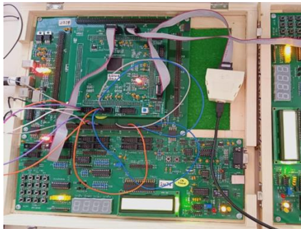
Fig. 5. Result of 8x8 Vedic multiplier on Spartan-6 FPGA kit
