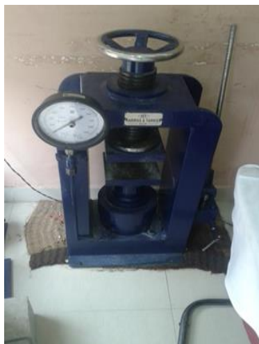
Fig. 4. Compressive strength testing machine
