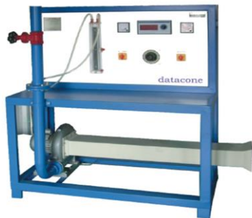
Fig. 1. Experimental Set-up of Pin Fin
