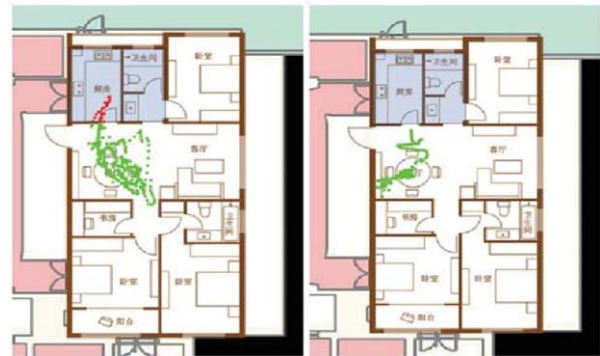
Fig. 12. False alarm rate experimental positioning data
