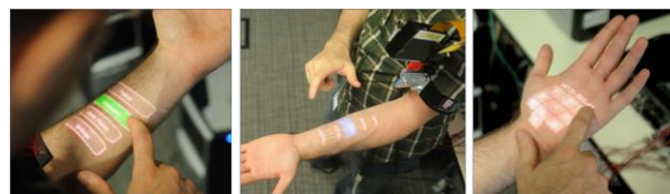
Fig. 11. Our sensing armband augmented with a pico-projector; this allows interactive elements to be rendered on the skin
