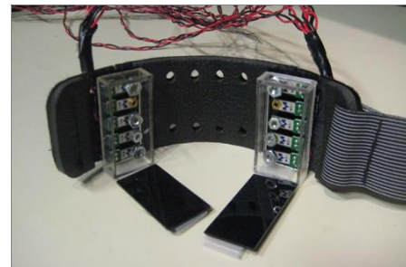
Fig. 1. A wearable, bio-acoustic sensing array built into an armband. Sensing elements detect vibrations transmitted through the body. The two sensor packages shown above each contain five, specially weighted, cantilevered piezo films, responsive to a particular frequency range.
