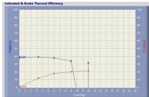
Fig. 4. Load vs. Indicated & Thermal Efficiency
