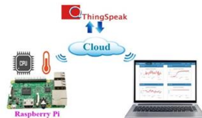
Fig. 13. Sensor data updated to Thing Speak cloud
