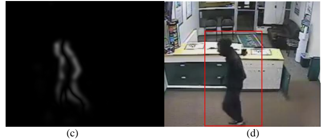
Fig. 3. (a) Previous frame (b) Current frame (c) Absolute Difference (d) Tracking
