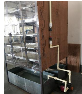
Fig. 13. Installation of rotameter and motor
