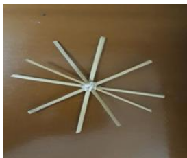
Fig 3. Radial mesh reinforcement
