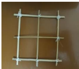
Fig. 2. Square mesh reinforcement
