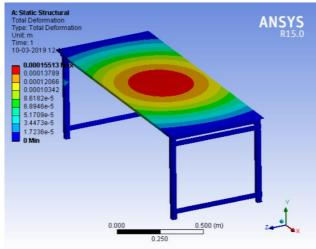
Fig. 14. Total Deformation of 100kg
