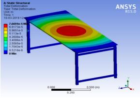
Fig. 12. Total Deformation of 25kg
