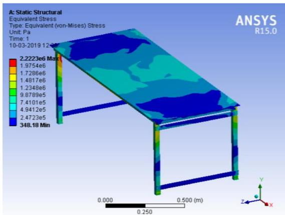
Fig. 13. Von-Mises Stress of 25kg
