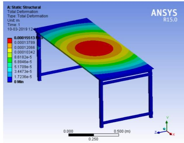
Fig. 14. Total Deformation of 100kg
