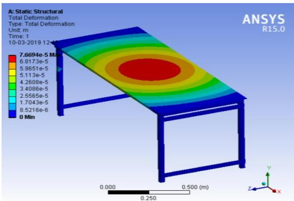
Fig. 12. Total Deformation of 25kg
