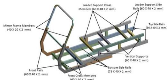
Fig. 1. Baseline design of vehicle chassis
