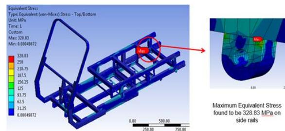
Fig. 10. Maximum equivalent stress was found to be 328.83 MPa
