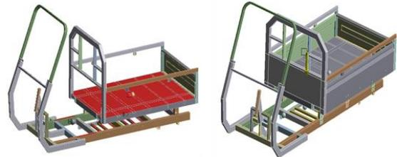
Fig. 7. Load of 10,000 N (1 tonne) applied on the carrier & Point Mass of 120 kg applied on the front driver seat area
