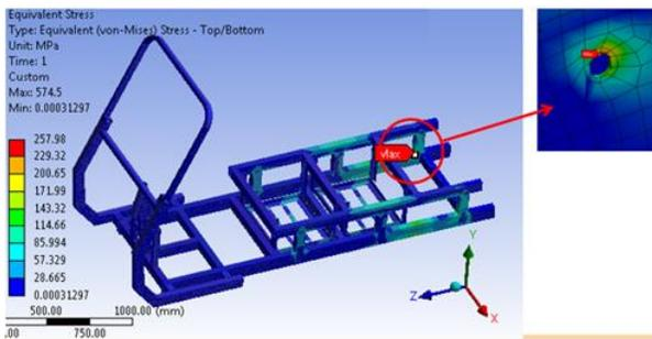
Fig. 14. Maximum equivalent stress was found to be 328.83 MPa
