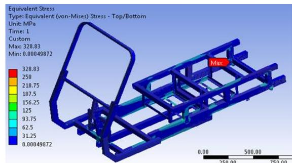
Fig. 9. Maximum equivalent stress was found to be 328.83 MPa
