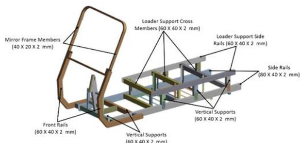
Fig. 2. Modified design of vehicle chassis
