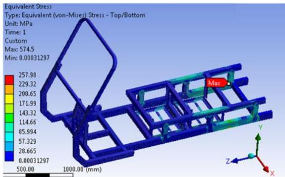
Fig. 13. Maximum equivalent stress was found to be below 240 MPa
