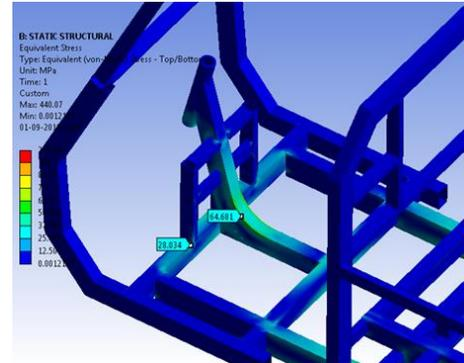
Fig. 15. Stress distribution at front handle location, stress has decreased in modified Design
