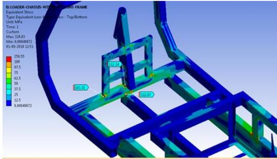
Fig. 11. Maximum equivalent distribution plot near front suspension location
