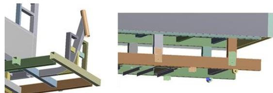
Fig. 8. Front suspension and rear leaf spring eyes surface are assigned as fixed support in all the directions
