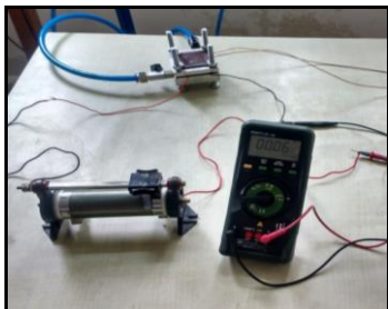
Fig. 6. Thermoelectric generator connected with multi-meter and rheostat
