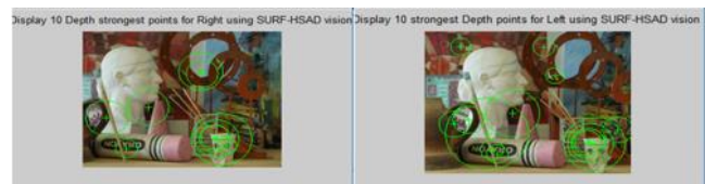
Fig. 4. Display of strong depth points in right and left stereo images using openSURF algorithm
