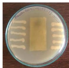
Escherichia coli ATCC 25922 Staphylococcus aureus ATCC 6538 Fig. 8. Assessment of qualitative antibacterial activity of Thulasi NPs finished fabric (BEFORE WASH)
