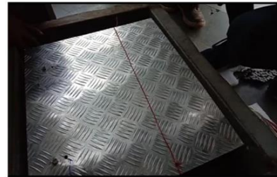
Fig. 7. Speed breaker when the speed is within the limit
