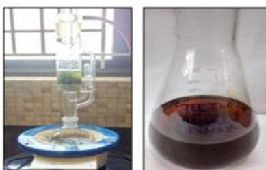
Fig. 2. Soxhlet extraction process of Appakovaithalai
