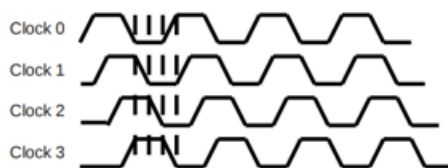
Fig. 1. The four shifted clock signals
