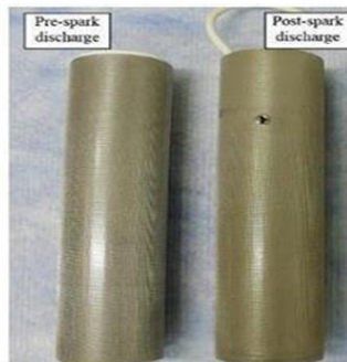
Fig. 2. Filter damage due to cathodic hotspot [1].
