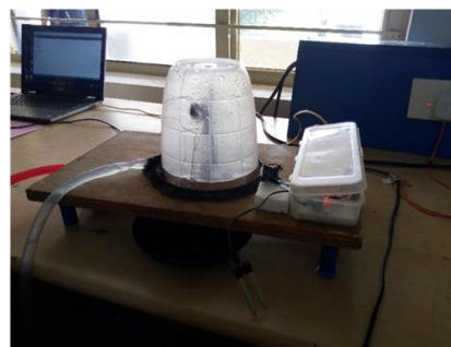
Fig. 3. Prototype of smart atomizer system using IoT
