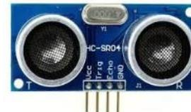
Fig. 5. Ultrasonic Sensor
