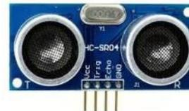
Fig. 5. Ultrasonic Sensor
