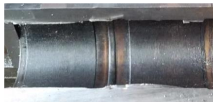
Fig. 3. Root penetration of Orbital Hot Wire TIG
