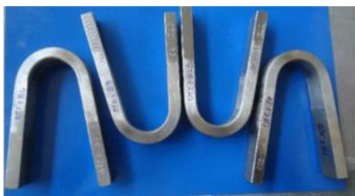
Fig. 7 (b). Bend Test Specimens
