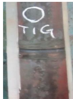
Fig. 2. Pipes welded using the Hot Wire Orbital TIG
