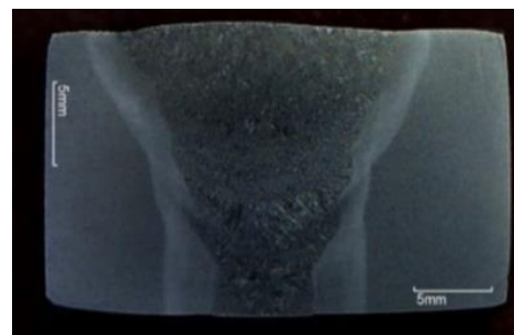
Fig. 4. No defect- OHW GTAW with normal Post weld heat treatment
