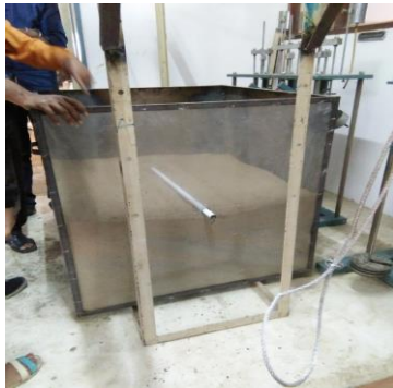
Fig. 4. Installation of nail
