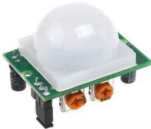
Fig. 8. PIR motion sensor
