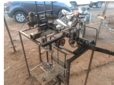
Fig. 1. Bar Cutting with Bending Machine
