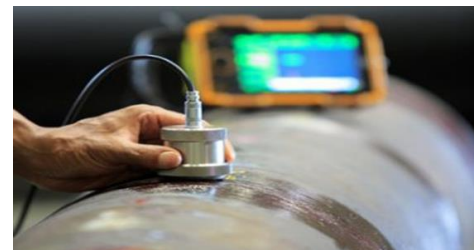
Fig. 2. Set up of ultra-sonic testing
