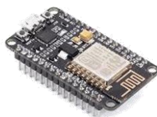
Fig. 6. ESP8266 based Node MCU development board
