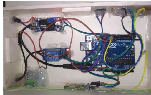
Fig. 12. Internal Circuitry of Android Based Security lock system with Password Reconfigurable option using Bluetooth and Microcontroller
