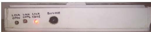
Fig. 11. Status Led's with Buzzer for user to know the status of the device and alert during wrong password entries.
