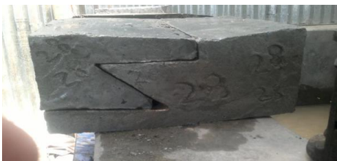
Fig. 3. Interlocked Sample 'a' loaded parallel to bed-plane for Crushing strength
