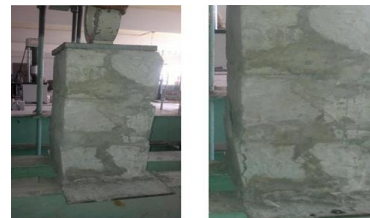
Fig. 6. Prism wall with using mortar for interlocking before and after cracking (Sample —b)
