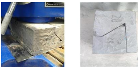
Fig. 4. Interlocked Sample 'b' loaded parallel to bed-plane for Crushing strength
