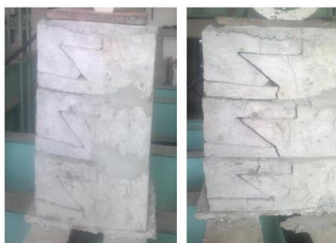
Fig. 5. Prism wall without using mortar for interlocking before and after loading Sample 'a'
