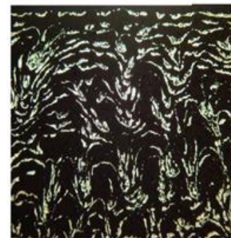
Fig. 3. Transparent concrete when optical fibers are in organic distribution
