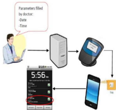
Fig. 2. NFC tag-based alarm activation for medical appointment.
