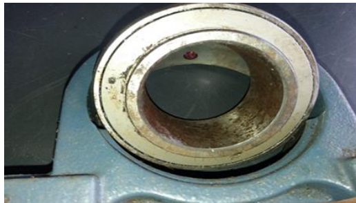
Fig. 9. Damage to Bering
