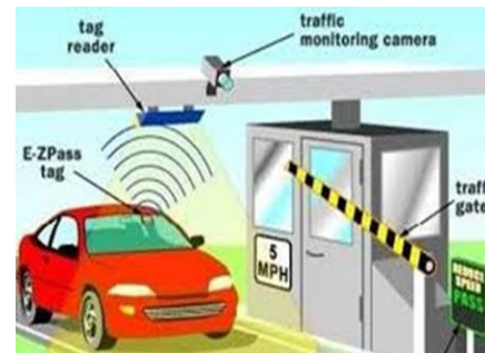
Fig. 1. RFID based toll gate collection
