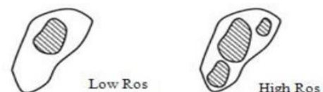
Fig. 2. Illustration of report between empty surface and total surface (Porosity) (Source: Huang J and all)
