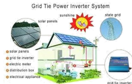
Fig. 1. Grid tie inverter system
