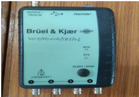
Fig. 2. FFT analyzer with four channels
