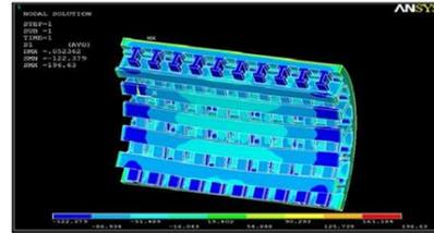
Fig. 6. Result of 1st Principle Stress of I- section (Aluminum)
