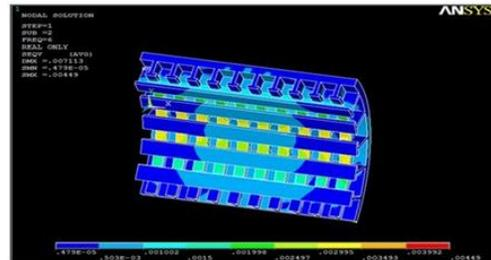
Fig. 12. Result of von mises stress of t- section (aluminum material)
