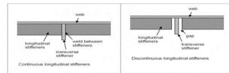
Fig. 2. (b) Continuous and Discontinuous longitudinal stiffeners
