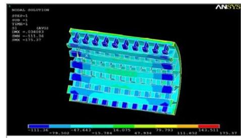
Fig. 7. Result of 1st Principal Stress of T- section (Carbon Fiber)
