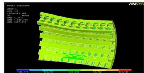
Fig. 9. Result of 2nd Principle Stress of I– Section (Aluminum Material)
