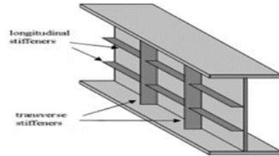
Fig. 2. (a) Stiffeners on I-section grid
