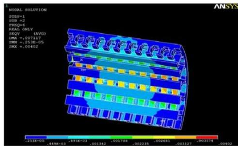
Fig. 13. Result of Von mises stress of I- Section (Aluminum Material)
