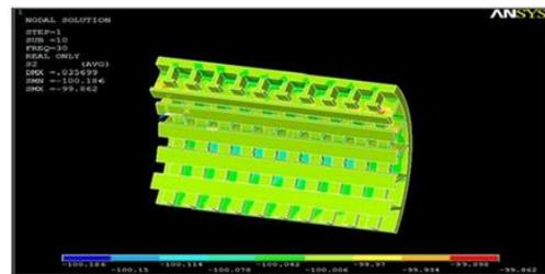
Fig. 8. Result of 2nd Principle Stress of T – Section (Aluminum Material)
