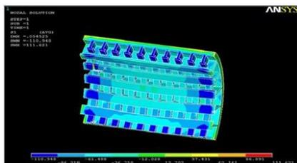
Fig. 5. Result of 1st principle stress of T-section (Aluminum)
