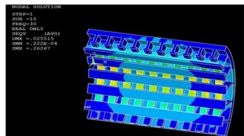
Fig. 14. Result of Von mises stress of T- Section (Carbon Fiber Material)
