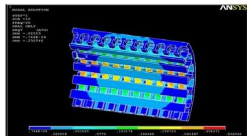
Fig. 15. Result of Von mises stress of I- Section (Carbon Fiber Material)
