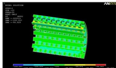
Fig. 10. Result of 2nd Principle Stress of T– Section (Carbon Fiber Material)
