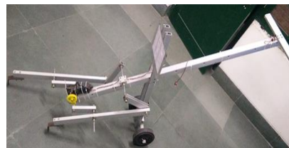
Fig. 2. Battery operated agriculture weeder
