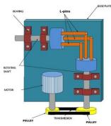
The mechanism is made of SRRS pair (sliding revolute sliding) sliding pair between the input hub hole and the link; revolute pair between link and input hub; revolute pair between link and output hub; sliding pair between holes in output hub and the link. The rotational motion of input shaft is converted into sliding motion of links which is then converted to rotational motion of the output shaft.
