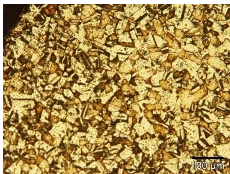
Fig. 15. Microstructure after final pillgaring outside tube
