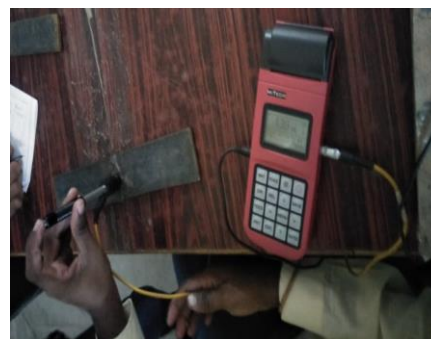
Fig. 2. Performing leeb hardness test
