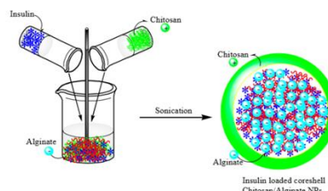
A schematic showing the preparation of chitosan-alginate NPs incorporating insulin.
