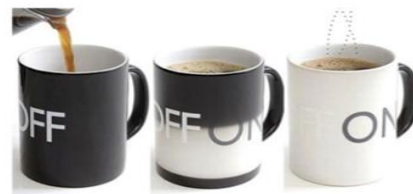
Fig. 1. The black pigment turns transparent when a heat source is applied
