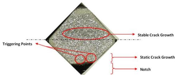
Fig. 17. SSCN specimen with static and stable crack growth.
