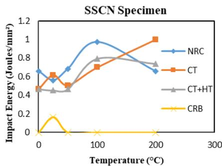
Fig. 19. Impact Energy vs. Temperature of SSCN specimen.
