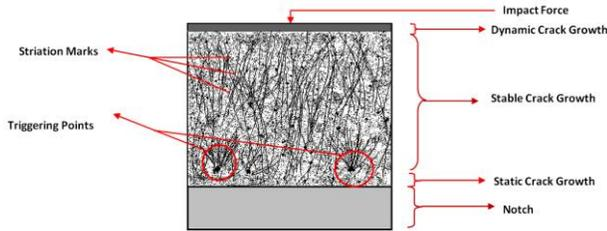
Fig. 30. SSFN specimen with dynamic, static and stable crack growth.
