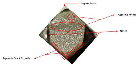
Fig. 21. DSCN specimen with dynamic crack growth
