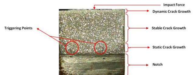
Fig. 29. SSFN specimen with dynamic crack growth.
