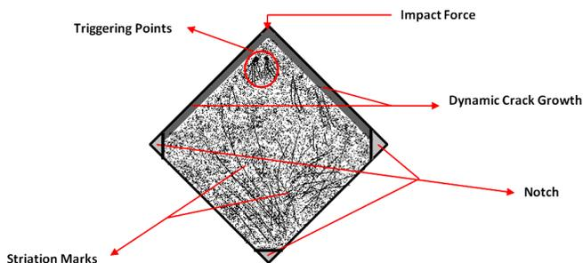
Fig. 26. TSCN specimen with dynamic, static and stable crack growth.
