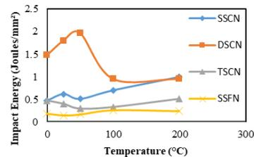
Fig. 9. Effect of coating on Impact Energy in different notch oriented specimens.
