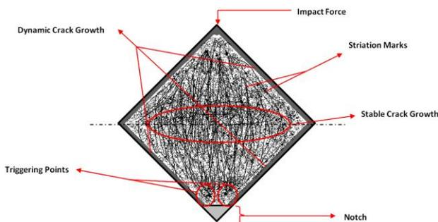
Fig. 18. SSCN specimen with dynamic, static and stable crack growth.
