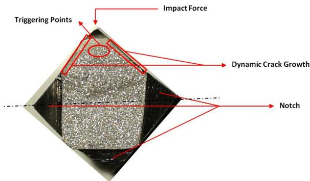
Fig. 25. TSCN specimen with dynamic crack growth.
