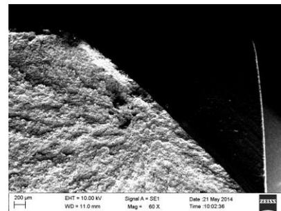
Fig. 15. SEM image of triggering points in SSCN specimen.
