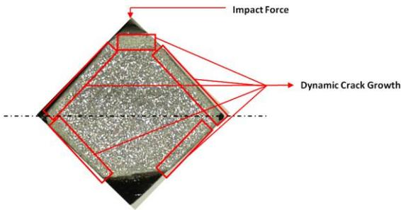
Fig. 16. SSCN specimen with dynamic crack growth.
