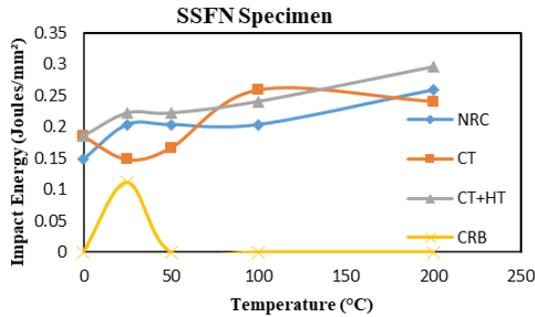
Fig. 31. Impact Energy vs. Temperature of SSFN specimen.
