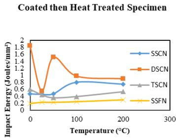
Fig. 11. Effect of coating then heat treating on Impact Energy in different notch oriented specimens.
