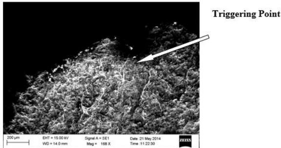
Fig. 24. SEM image of triggering points in TSCN specimen.
