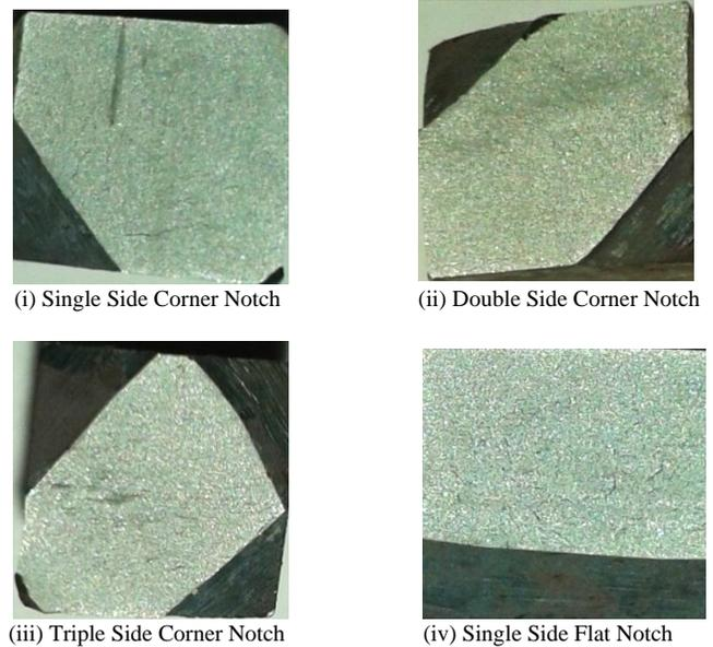
Fig. 14. Fractured surface of SSCN, DSCN, TSCN, and SSFN specimen in carburized condition.
