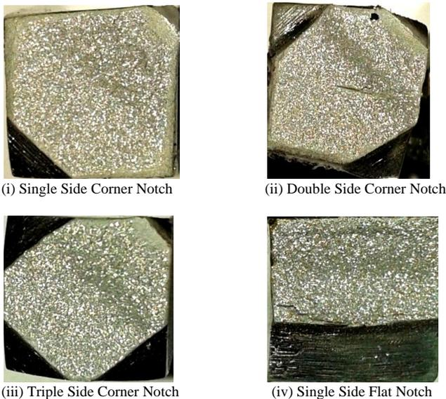
Fig. 12. Fractured surface of SSCN, DSCN, TSCN, and SSFN specimen in coated then heat treated condition.
