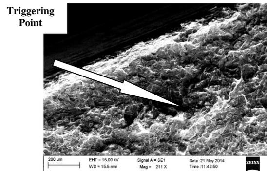
Fig. 28. SEM image of triggering points in SSFN specimen.
