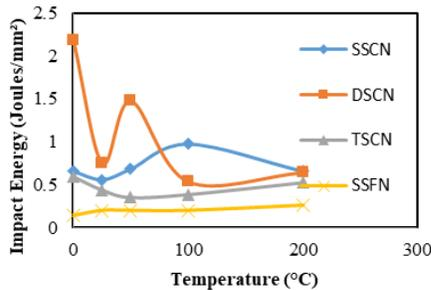
Fig. 7. Effect of normal condition on Impact Energy in different notch oriented specimens.
