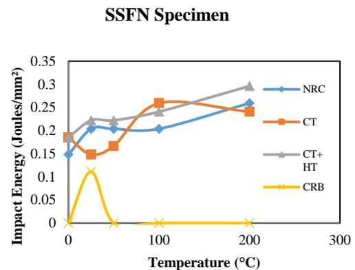
Fig. 5. Effect of service temperature of SSFN specimen on Impact Energy.
