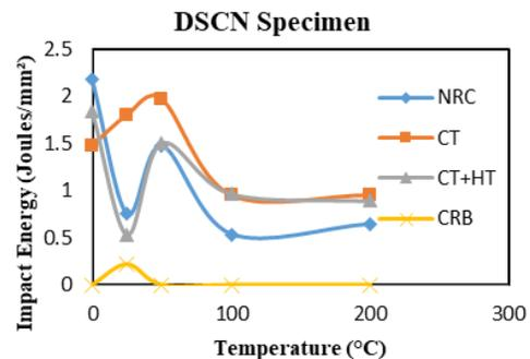
Fig. 23. Impact Energy vs. Temperature of DSCN specimen.
