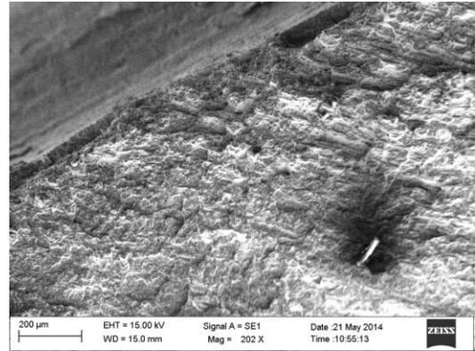
Fig. 20. SEM image of triggering points in DSCN specimen.
