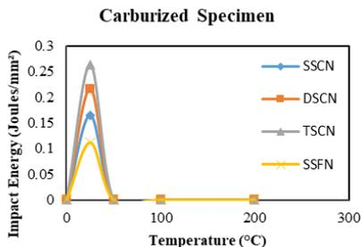
Fig. 13. Effect of carburized on Impact Energy in different notch oriented specimens.
