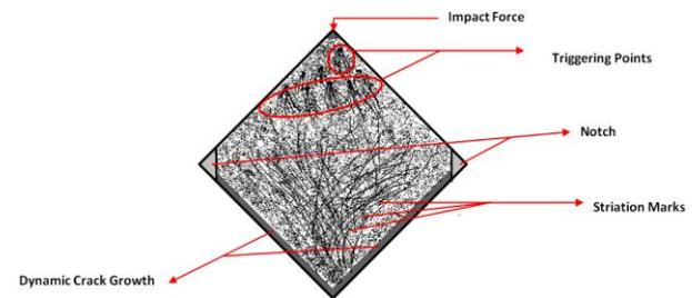
Fig. 22. DSCN specimen with dynamic, static and stable crack growth.
