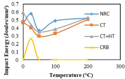
Fig. 27. Impact Energy vs. Temperature of TSCN specimen.
