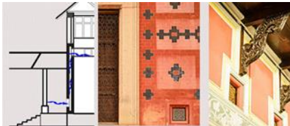
Fig. 6. Double wall with cavity
